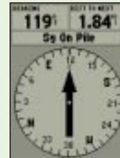
The navigation page displays the direction, bearing and distance to your destination.
