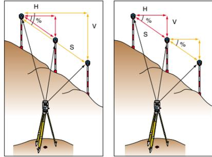
At the touch of a key, the Series 10 measures horizontal distance, slope distance, height difference and percentage of slope between two prisms.
