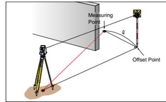
The Series 10 calculates the angles and distance, or the coordinates of the measuring point by inputting the distance and direction between the measuring point and the offset prism.
