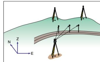
The Series 10 performs three-dimensional setting out with N, E and Z or E, N and Z coordinates. Directions and distances to the setting out position are indicated on the screen.
