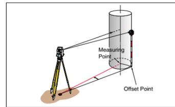
The Series 10 automatically calculates the position of measuring points. First, set the prism on either side of the measuring point at the same distance from the Series 10 instrument. Measure the prism, then sight the measuring point.
