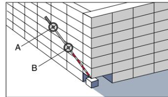
The Series 10 calculates the position of the measuring point in angles and distance, or in coordinate values.
