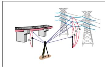
The Series 10 easily determines the height of a point where a prism cannot be placed. Sight a prism either directly above or directly below the target point, and then sight the target point.
