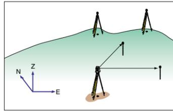
The Series 10 calculates 3-D coordinate values of measuring points and displays them either as N,E,Z or E,N,Z.
