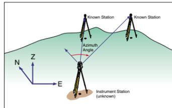
When using three or more points, the distance is not required. Station elevation from known reference points (up to 10 points) can also be calculated and each deviation of multiple reference points is displayed. If a bad point is selected it can be recalculated, re-observed or replaced with a new point.
