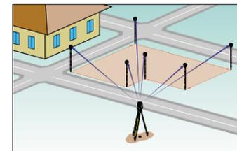
The Series 10 can use measured points or stored data to calculate an area.
