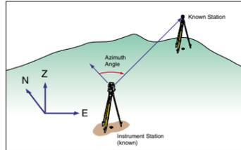
The Series 10 can automatically set the horizontal angle to the azimuth of a back sight by using the coordinates of the instrument station and the back sight point.
